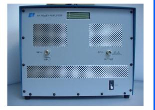
The 1140LA Amplifier is a rugged source of RF power for ultrasonics, induction heating and laser modulation as well as plasma applications. It is a totally solid state solution employing RF DMoS FETs in the power amplification stages, offering simultaneous forward and reverse power readouts, and RS232 port for data collection. The 1140LA reflects E&I's commitment to reliable and robust RF power.
