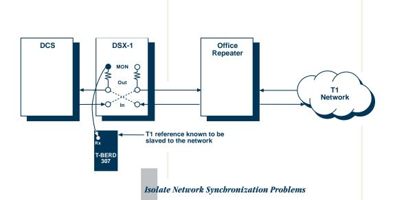
Timing problems are easily identified. Compare T1 circuit against a network reference clock to isolate timing slips.
