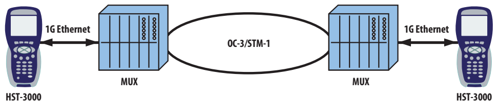
Figure 2. Class-of-service testing using the HST-3000 Ethernet SIM with the Multiple Streams option
