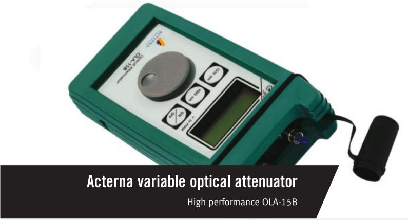
The Acterna OLA-15B is a handy-sized, rugged optical attenuator for single mode applications from 1260 to 1625 nm. Applications include bit error rate tests, determination of system margin and receiver sensitivity, and calibration of optical power meters.
