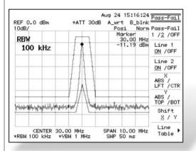
Any UPPER and LOWER limit lines can be set. Pass or Fail judgement can be made in accordance with the limit lines.
