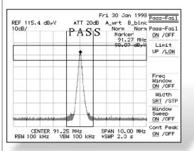
The window range set along the X and Y axes is the PASS area. The signal level or frequency at a marked point is evaluated in accordance with the range.
