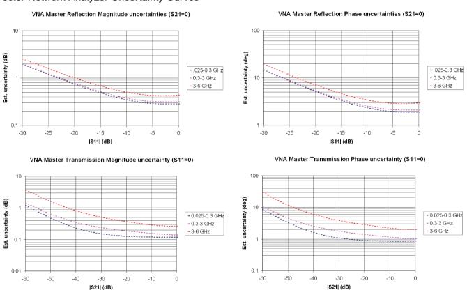
The uncertainty graphs above provide measurement uncertainty at 23° C after vector correction for the standard N connector type. Errors are worse-case contributions of residual directivity, source match, frequency response, network analyzer dynamic range, and connector repeatability. For the 1-path 2-port measurements, transmission tracking, crosstalk and physical load match termination was added. OSLN50-1 calibration components were used.
