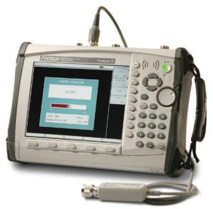
The easy-to-view Power Monitor display minimizes keystrokes when testing in the field.
