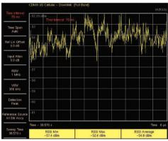
With Option 25, RSSI measurement analyzes signal strength of a signal over time.
