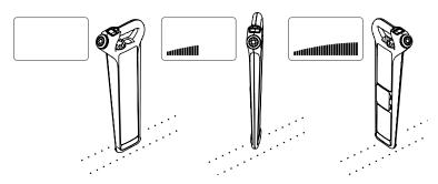
Trace the buried conductor keeping the C.A.T4 vertical and moving it steadily from side to side. Follow the line of the buried conductor, marking it as required across the area to be excavated.
