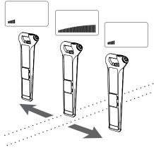
and forth across the maximum readout position, the cable or pipe's position can be pinpointed. The tidemark feature hold the maximum bargraph reading to ease identification of a peak readout.
