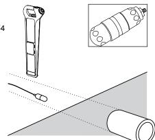
Smaller ghost signals appear before and behind the main signal position. Locate all three peaks to be sure the largest middle one is identified as the Mouse position.
