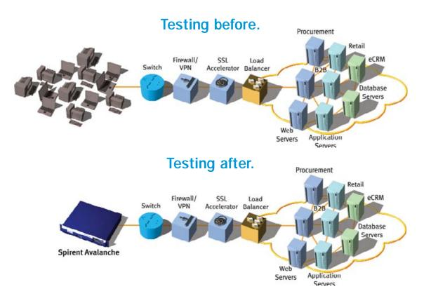
The Spirent Communications Reflector test appliance is a companion solution designed to simulate large Web, mail and streaming server infrastructures. When used together, Avalanche and Reflector provide an ideal testing strategy for enterprise network operators, equipment manufacturers and service providers. This two-pronged approach delivers a reliable, quantifiable way of establishing performance thresholds, and can be used to test both individual devices and networks to capacity.
