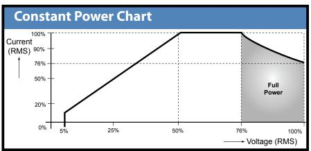
Note: Constant power mode provides increased current at reduced voltage. Maximum available current shown.
