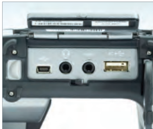
From Left to right: USB mini for PC image download, 4 pole audio for voice annotation, NTSC video, USB-A for memory stick image transfer
