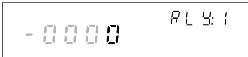
Relay status display for Relay 1 (for example 1111-0000)
