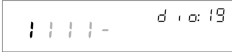
Digital I/O status display for DIO line 19 (for example 1111-0000-0000-0000)
