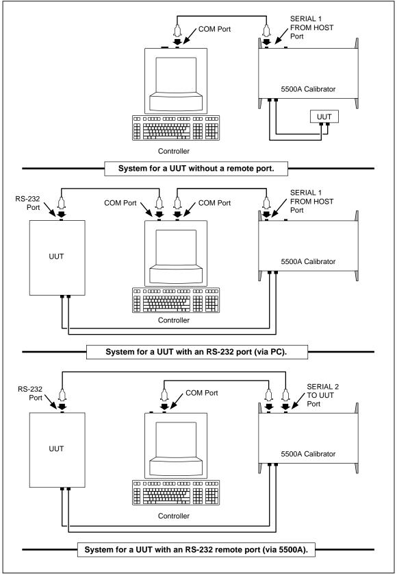
Figure 5-2. Typical RS-232 Remote Control Connections
