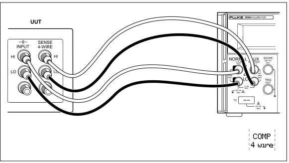
Figure 4-4. UUT Connection: Capacitance (Four-Wire Compensation)
