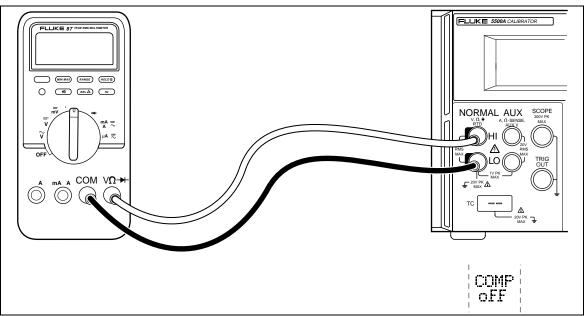
Figure 4-6. UUT Connection: Capacitance (Compensation Off)
