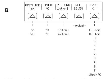
TYPE selects the thermocouple type that you are measuring (factory default is K); REF is the actual temperature of the reference source; REF SRC is the reference temperature, the internal 5500A Calibrator reference (intrnl) or an external reference (extrnl) (factory default is intrnl); UNITS selects °C or °F; OpenTCD selects the open thermocouple detector feature (default on).
