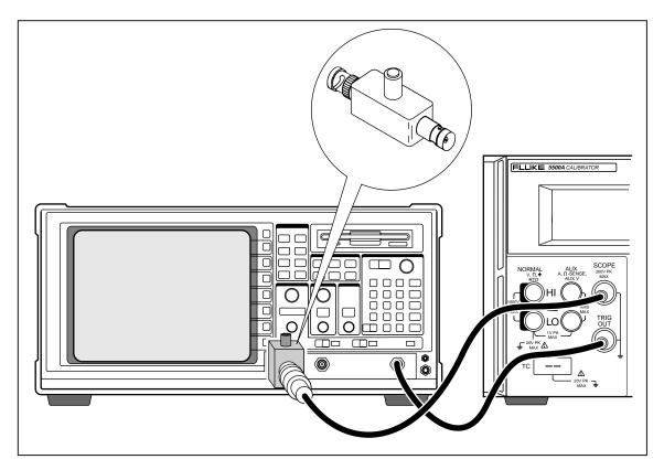
Figure 8-2. Tunnel Diode Pulser Connections
