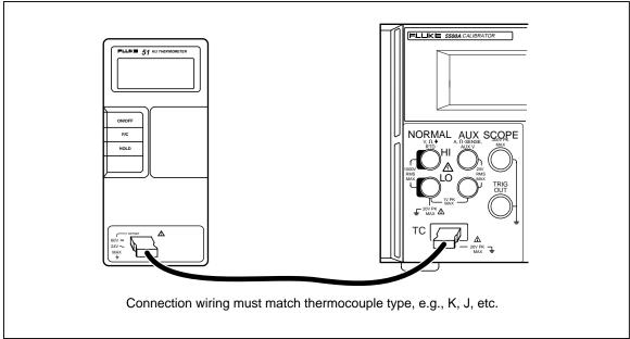
Figure 4-10. UUT Connection: Temperature (Thermocouple)
