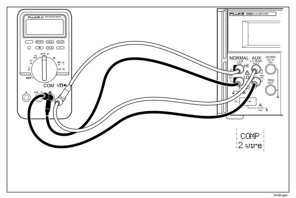
Figure 4-5. UUT Connection: Capacitance (Two-Wire Compensation)
