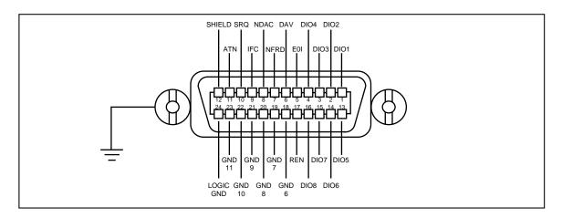
Figure C-1. IEEE-488 Connector Pinout (connection side)
