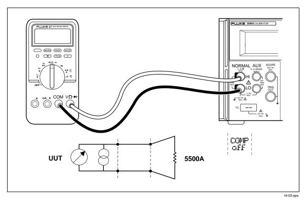
Figure 4-3. UUT Connection: Resistance (Compensation Off)
