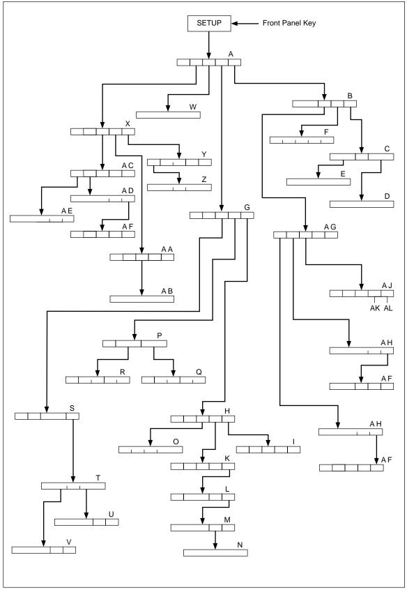
Figure 3-3. SETUP Softkey Menu Tree
