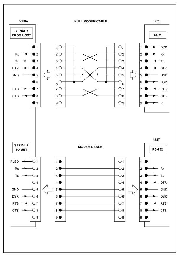
Figure C-4. Serial Port Connections (DB-9/DB-9)
