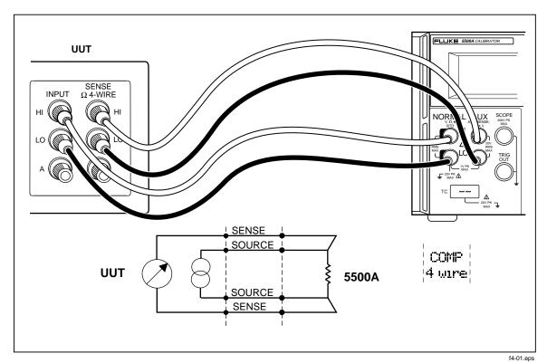
Figure 4-1. UUT Connection: Resistance (Four-Wire Compensation)
