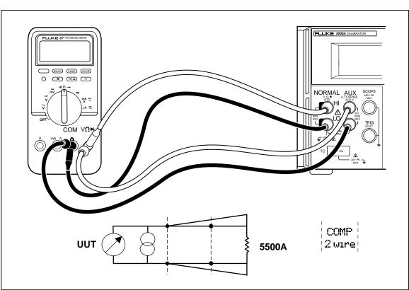
Figure 4-2. UUT Connection: Resistance (Two-Wire Compensation)
