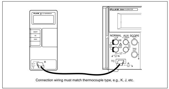
Figure 4-19. Cable Connections for Testing a 50 Series Thermometer
