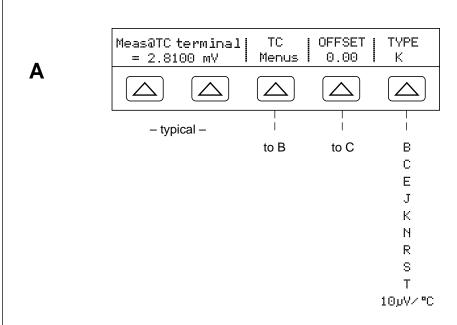
TYPE selects the thermocouple type that you are measuring; OFFSET enters a temperature offset; TC Menus selects more setup parameters; Meas@ TC terminal is the actual input voltage from the thermocouple being measured.
