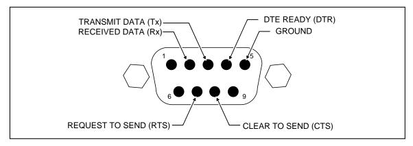
Figure C-2. SERIAL 1 FROM HOST Port Connector Pinout
