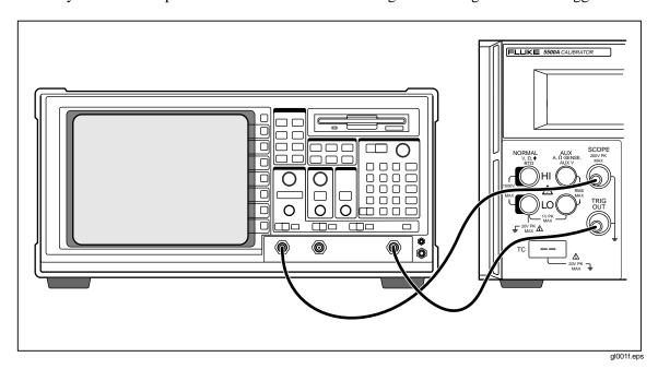
Figure 8-1. Oscilloscope Connection: Channel and External Trigger
