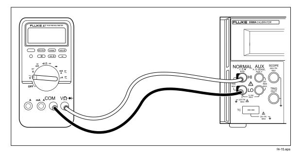
Figure 4-15. Cable Connections for Testing an 80 Series General Functions
