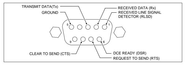
Figure C-3. SERIAL 2 TO UUT Port Connector Pinout (connection side)
