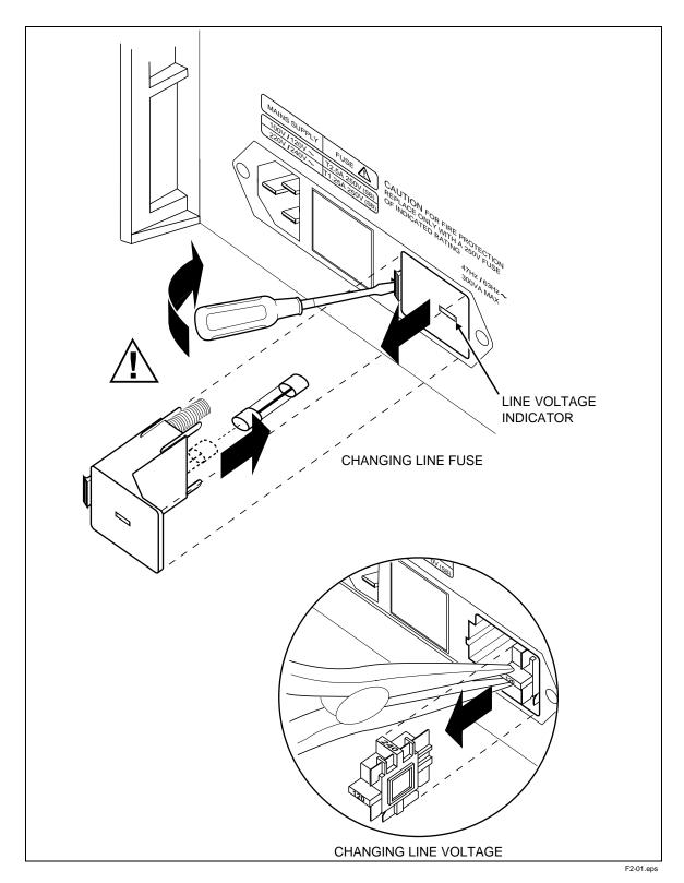
Figure 2-1. Accessing the Fuse and Selecting Line Voltage
