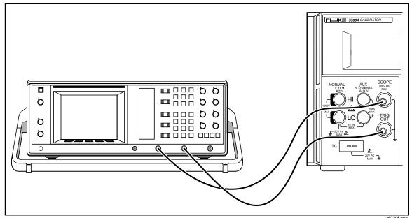
Figure 8-3. Oscilloscope Connection: Channel and External Trigger
