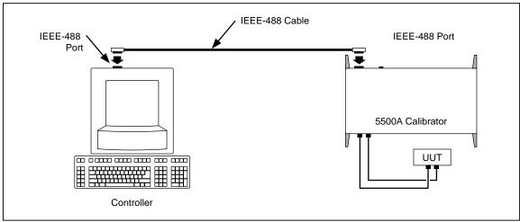
Figure 5-3. Typical IEEE-488 Port Connections
