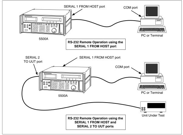
Figure 1-2. RS-232 Remote Connections
