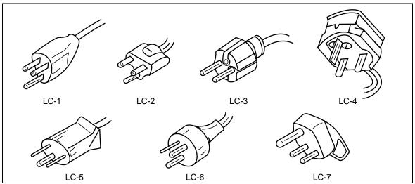
Figure 2-2. Line Power Cord Types Available from Fluke
