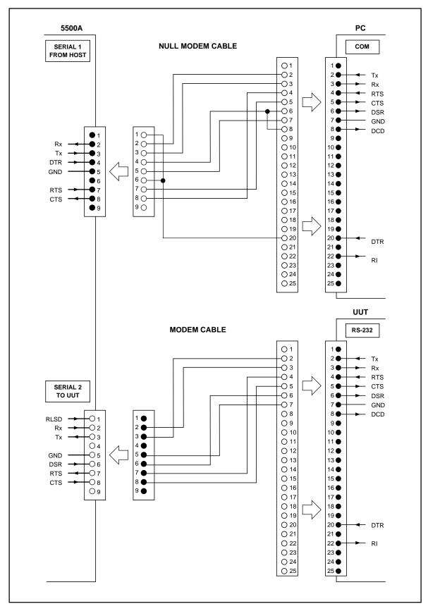
Figure C-5. Serial Port Connections (DB-9/DB-25)
