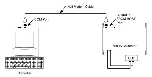
Figure 5-4. Typical PC COM Port Connections
