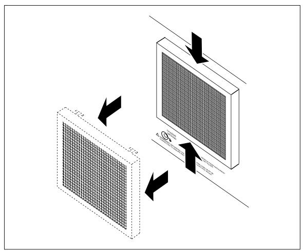
Figure 7-2. Accessing the Air Filter
