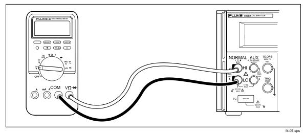
Figure 4-7. UUT Connection: DC Voltage/AC Voltage
