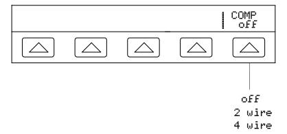
• **COMP** (Compensation) Applies 4-wire compensation, 2-wire compensation or turns compensation off. Compensation refers to methods of connecting the 5500A to the UUT to cancel out test lead resistance (NOT capacitance). Compensation is available for capacitances of 110 nf and above. This softkey will not function below 110 nf. See "Four-wire versus Two-wire Connections" earlier in this chapter for more information.
