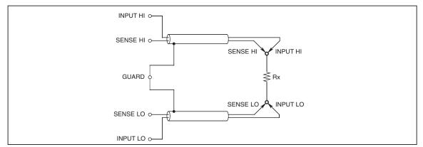
Figure 3-6. 4-Wire Measurements
