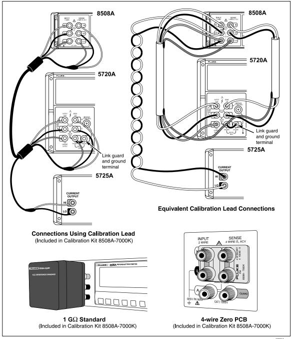
Figure 6-1. Equipment Connections Required for Calibration
