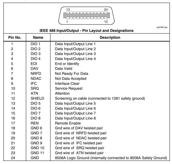
Figure 4-1. IEEE 488 Input/Output Connector
