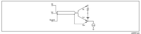
Figure 3-2. Twisted-Pair Cable Connections
