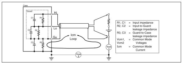
Figure 3-3. External Guard Connections
