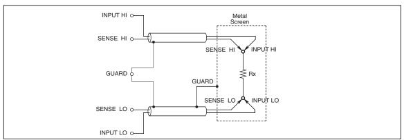
Figure 3-7. 4-Wire High Resistance Measurements
