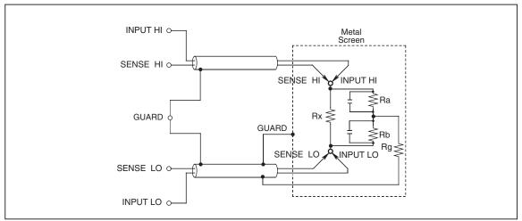
Figure 3-9.  $\Omega$  Guard Measurements
