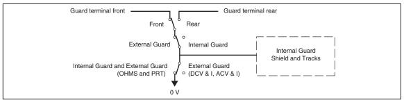
Figure 3-4. Internal Guard Connections
