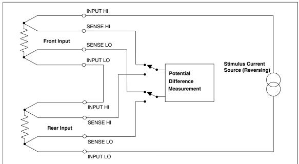
Figure 3-12. TruΩ Ratio Measurements
