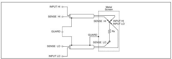
Figure 3-8. 4-Wire Resistance Zero Measurements
