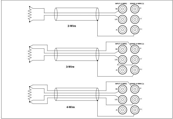
Figure 3-11. PRT Connections
