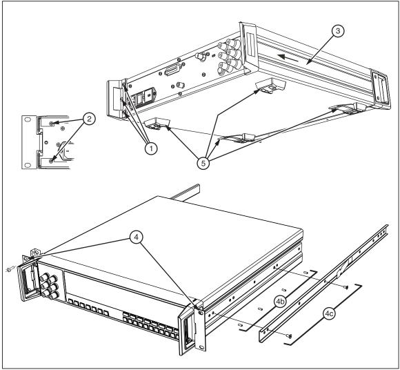
Figure C-1. Installing the 8508A Rack Mount Slide Kit
