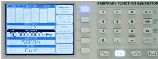
Fig. 4.3: Front view including display of the settings
