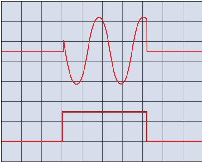
Fig. 7.2: Output signal controlled by a GATE signal
