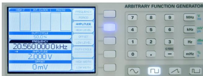
Fig. 4.5: Front view including display of the amplitude change
