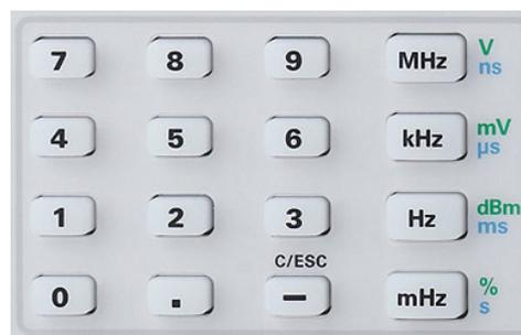
Fig. 4.2: numeric keypad and key's for unit's and escape
