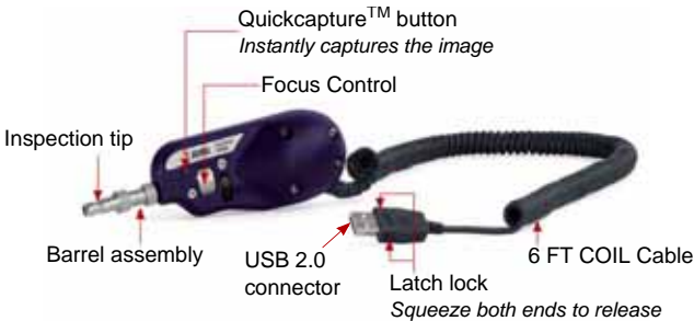
Fig. 16 P5000 Probe components
