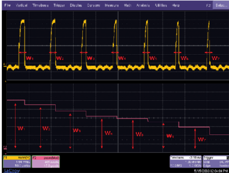
Example of how Modulation Analysis measures the width of individual pulses and displays their value on the vertical axis.
