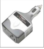
The inverter's output provides a true sine wave rated to deliver 60 watts of ac power continuously or 75 watts of power for 5 minutes. It is also protected with features that will automatically shut off in case of under-voltage, over-voltage, and over-temperature.
