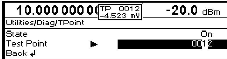
Fig. 4-41 Utilities – Diag – TPoint menu
