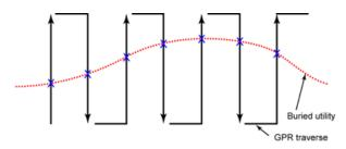
Figure 4.1: cross and mark surveying
