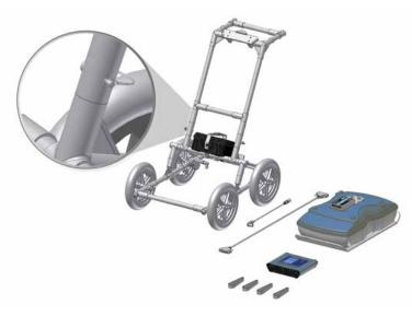
3. Attach the Sensor to the Cart using the Sensor Support Straps. Ensure the Sensor is oriented the correct way with the connections toward the back of the Cart. Using the Sensor Support Straps, adjust the height of the Sensor so it's  $1-2 \text{ cm} (\frac{1}{2} - \frac{3}{4} \text{ inch})$  above the ground.
