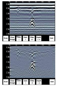
Figure 3.22: filter adjustments
