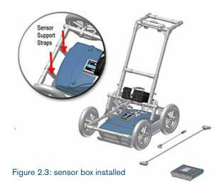
4. Attach the Display Unit to the Display Unit Mount on the Cart. Depress the flexible clip and slide the Display Unit back far enough so the clip catches and secures it firmly in place. Adjust the angle of the Display Unit by loosening the hand-screws underneath the Display Unit Mount, rotating the Display Unit to the desired angle and tightening the hand-screws. This ensures the Display Unit does not rotate and damage the Display Cable.
