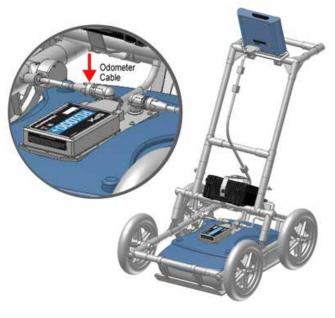
Figure 2.6: installing the odometer cable
