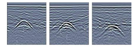
Figure 4.2: locating a concrete pipe
