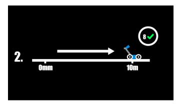
Roll the RD1000+ along the measured path; a red line rotates to indicate that the odometer is turning. Press '8' again when you get to the measured distance and the below screen will appear:
