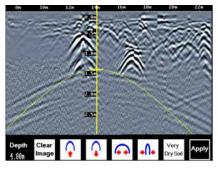
Figure 3.17: air wave reflections
