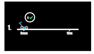
Align the RD1000+ at the start point and press '8' to begin the calibration. The following screen appears:
