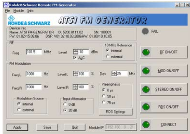
Fig. 2: R&S® ATSI100 module configuration software (R&S® ATSI100 FM generator)
