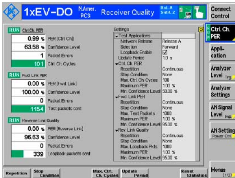
The receiver quality measurement display shows the key results regarding the mobile's receiver performance.
