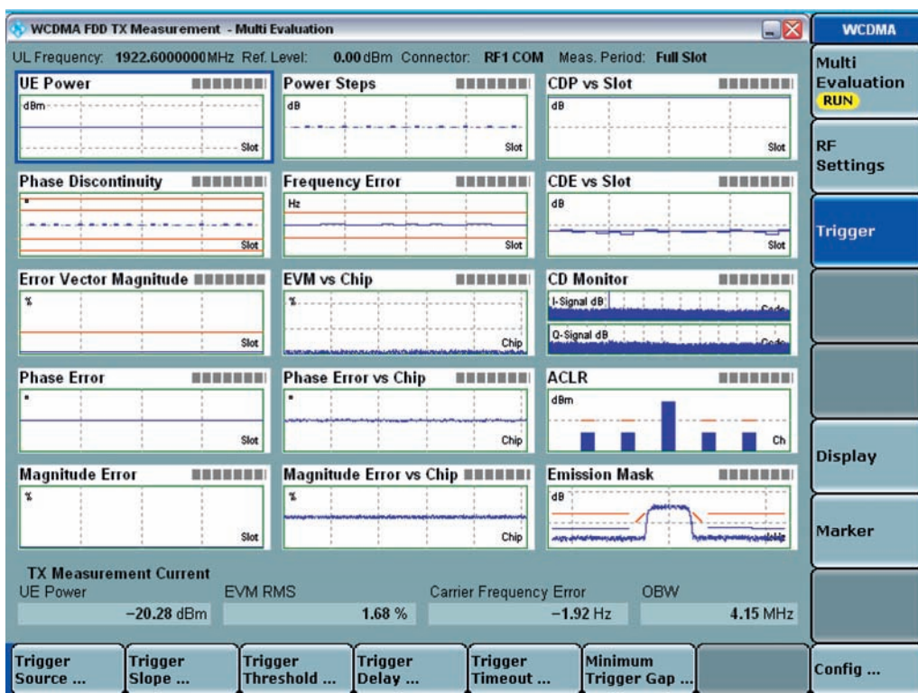
Overview screen: WCDMA TX measurement – R&S®Multi-Evaluation.
