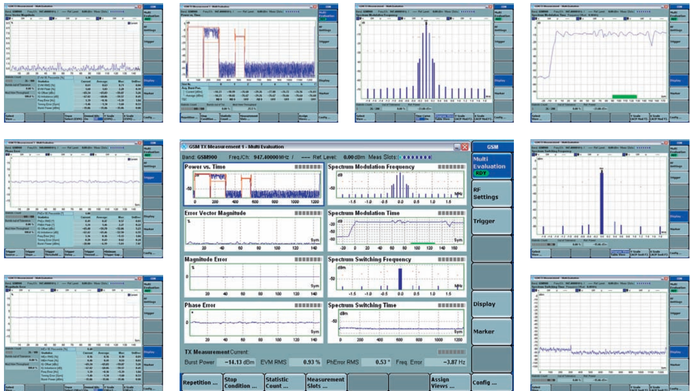
R&S®Multi-Evaluation: GSM TX measurement.
