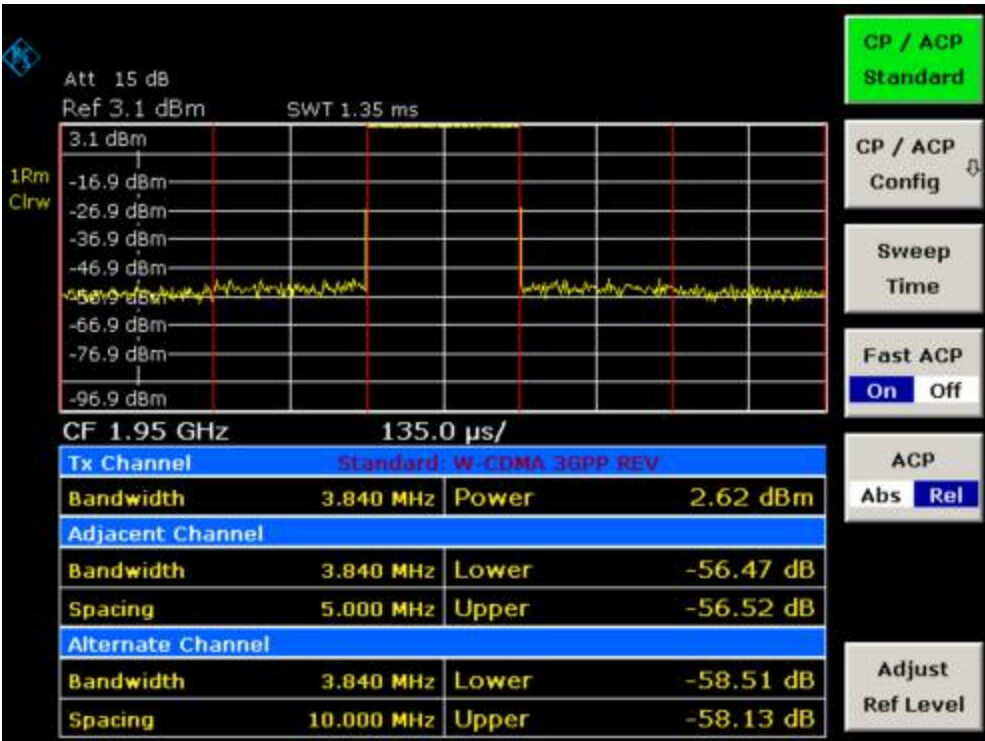
Fig. 2–25 Measuring the adjacent channel power of a W–CDMA signal with the fast ACP mode
