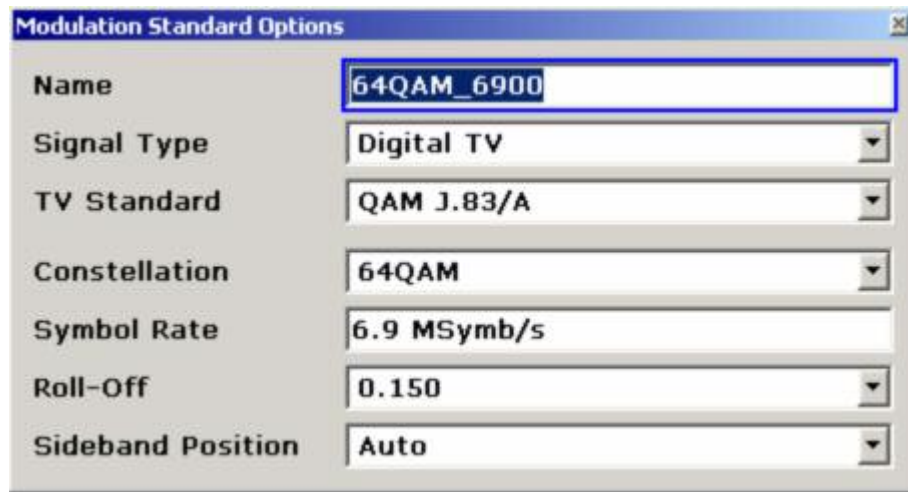
Fig. 2–48 Modulation Standard Options dialog box for digital TV
