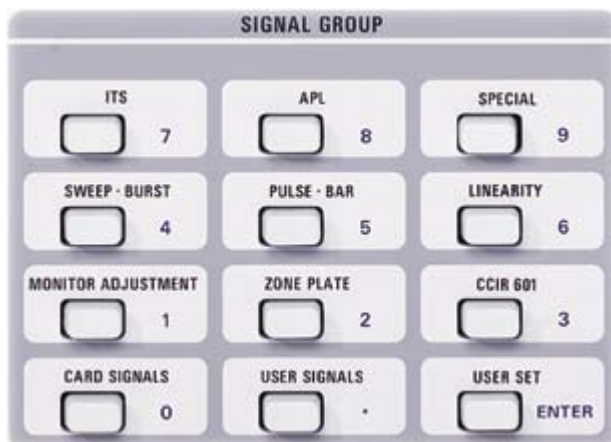
Twelve different signal groups can be called up via the front panel
