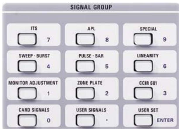
Twelve different signal groups can be called up via the front panel
