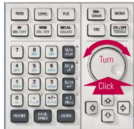
Rotary knob for menu navigation
