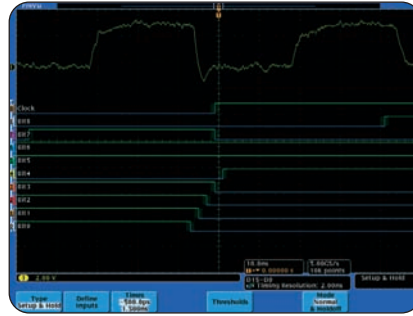
► Multi-channel setup-and-hold triggering highlighting multiple violations (MSO4000).
