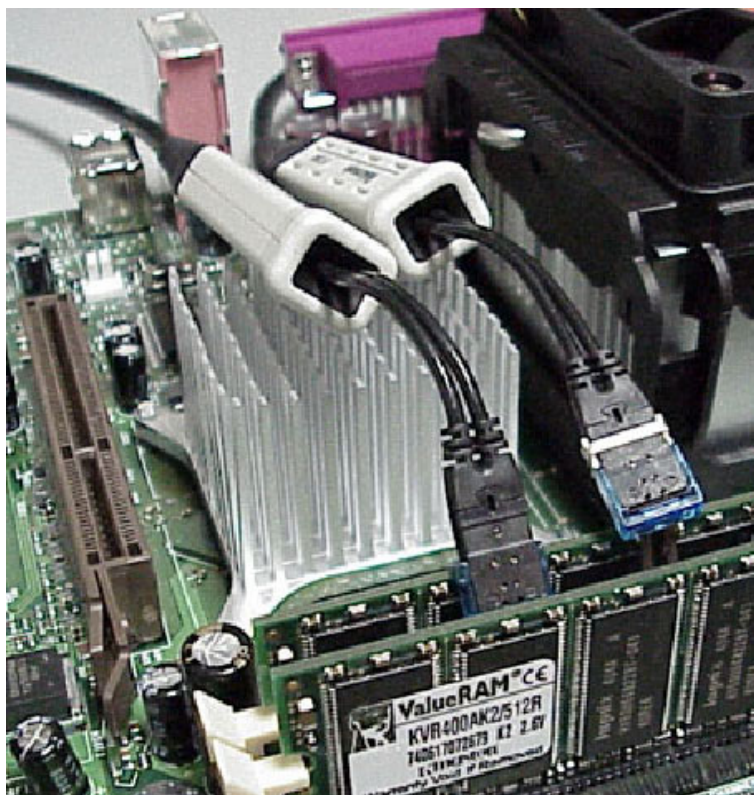
Figure 10: Soldered Tip-Clip assemblies
