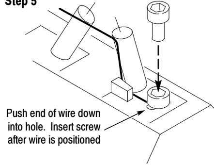
Push end of wire down into hole. Insert screw after wire is positioned
