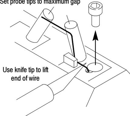
Use knife tip to lift end of wire
