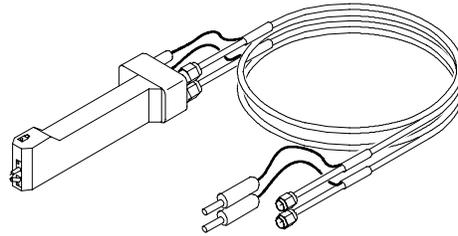
The P80318 probe is designed to be used with the Tektronix 80A02 EOS/ESD Protection Module. Together, they protect sensitive instrument-input stages, such as the sampling bridge of Tektronix electrical sampling modules, from electro-overstress (EOS) and electro static discharge (ESD) damage due to static charges stored in the device under test (DUT).
