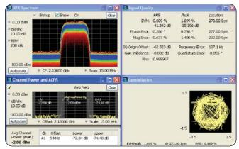
Time-correlated, multi-domain view provides a new level of insight into design or operational problems not possible with conventional analysis solutions. Here, ACLR and Vector Modulation Quality (Opt. 21) are performed on a single acquisition, combined with the continuous monitoring of the DPX spectrum display.
