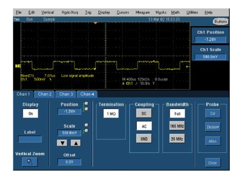
Figure 11: Typical waveform at AC Coupling
