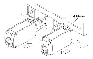
Figure 2: Connecting and disconnecting the TCA-1MEG
