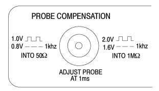
Figure 6: Probe Compensation Output of the TDS6604
