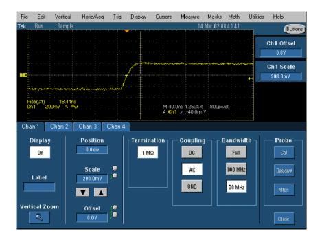
Figure 15: Typical waveform at 20 MHz bandwidth
