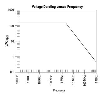
Figure 17: Voltage Derating versus Frequency
