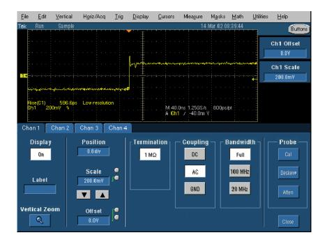
Figure 13: Typical waveform at Full (500 MHz) bandwidth
