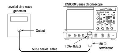
Figure 19: TCA-1MEG System Bandwidth equipment hookup
