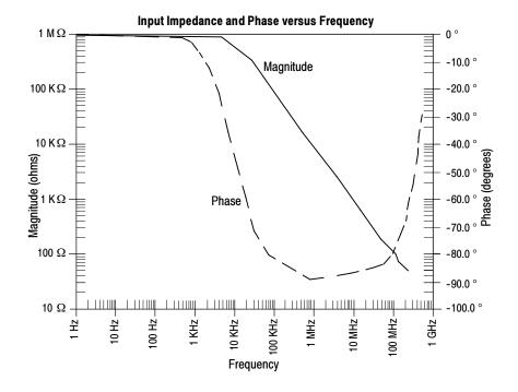
Figure 16: Typical Input Impedance and Phase versus Frequency
