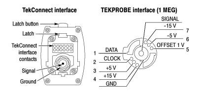
Figure 4: TekConnect and TEKPROBE Interface features
