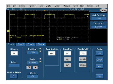
Figure 12: Typical waveform at DC Coupling
