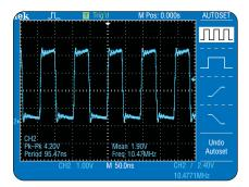
Automatically detects sine waves, square waves and video signals, with readouts of relevant measurements and additional user-selectable views of the signal.
