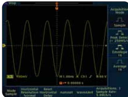
► The TDS3054B's 5 GS/s real-time sample rate and sin(x)/x interpolation ensure accurate reconstruction of a 500 MHz sine wave.
