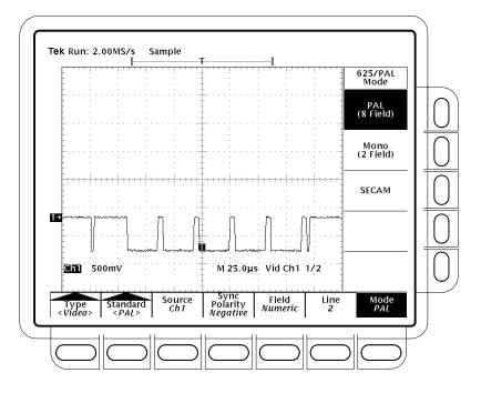
Figure 1–4: Video Trigger Menu — PAL Mode
