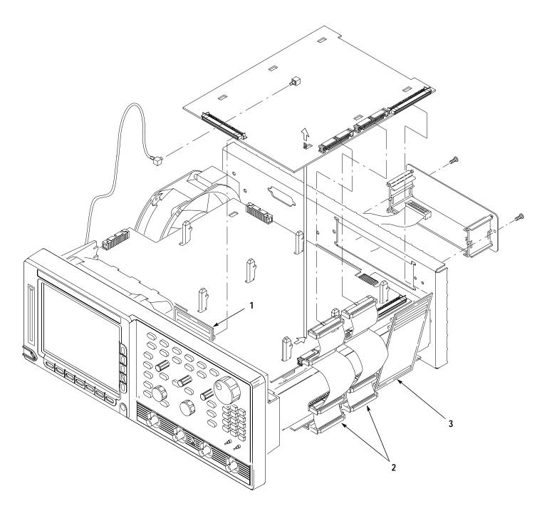
Figure 2–6: Circuit Board Removal
