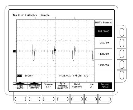
Figure 1–5: Video Trigger Menu — HDTV Format
