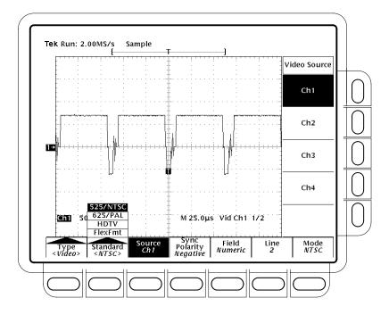
Figure 1–2: Video Trigger Menu — Standard
