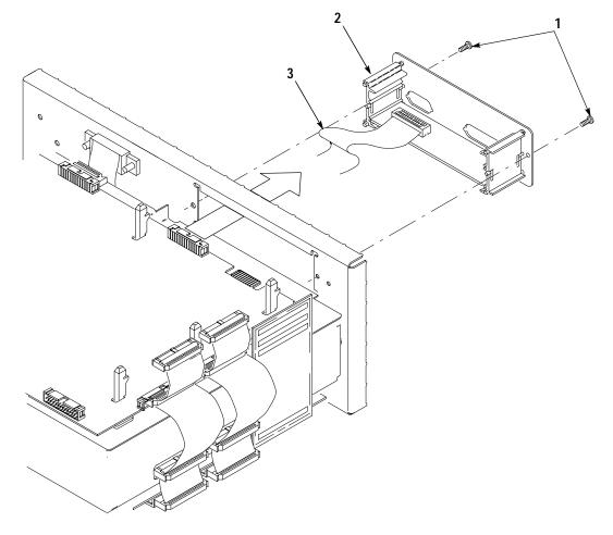
to remove the cable connector from the A23 SerPar board to the A11 Processor/Display board (see number 3 in Figure 2–4).
