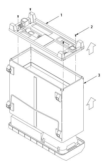
Figure 2–2: Rear Cover and Cabinet Removal
