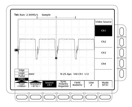
Figure 1–1: Main Trigger Menu — Video Type
