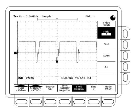
Figure 1–3: Main Trigger Menu — Field
