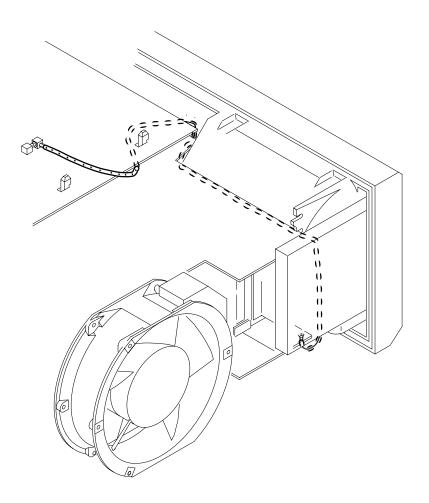
Figure 2–5: Proper Routing of the Video Cable
