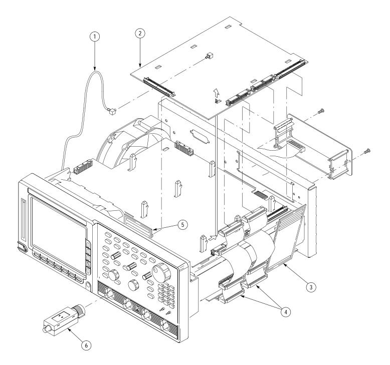
Figure 2–7: Video Trigger Replaceable Parts
