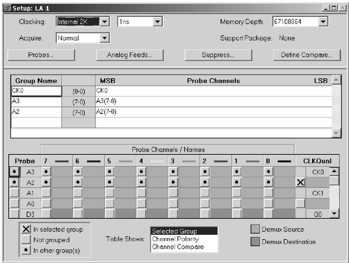
Figure 3- 16: Source and destination probe channels in Internal 2X Clocking mode
