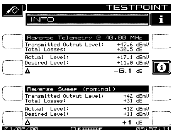
Fig. 4-4 Telemetry and Sweep Generation and Injection Levels
