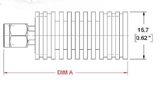
**Construction:** Black aluminum alloy body with passivated stainless steel connectors. Gold plated beryllium copper contacts.
