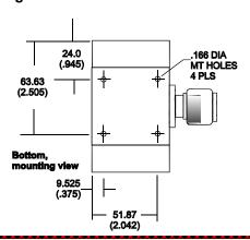
**Construction:** Black aluminum alloy body with passivated stainless steel connectors. Gold-plated beryllium copper female contact, stainless steel or gold-plated beryllium copper male contact.
