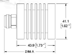
**Construction:** Black aluminum alloy body with passivated stainless steel connectors. Gold plated beryllium copper female contacts, stainless steel male contacts.
