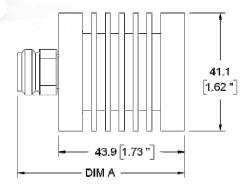
**Construction:** Black aluminum alloy body with passivated stainless steel connectors. Gold plated beryllium copper female contacts, stainless steel male contact.
