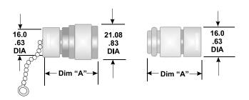
Construction: Passivated stainless steel body and connectors. Stainless steel male contact.
