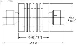
**Construction:** Black aluminum alloy body with passivated stainless steel connectors. Gold plated beryllium copper contacts.
