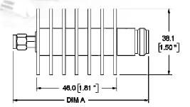
**Connectors:** Type N or SMA stainless steel M/F connectors per MIL-STD-348A, interface dimensions mate nondestructively with MIL-PRF-39012. Designed to meet MIL-DTL-3933 environmental specification. High power input is unidirectional: Input connector optional; Female if not specified.
