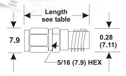
**Construction:** Passivated stainless steel body and connectors. Gold plated beryllium copper contacts.
