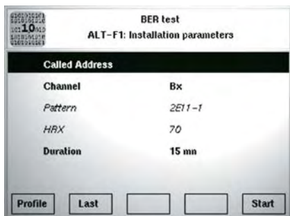
figure 6 After customization. Example: The automatic test checks the configuration of an access in accordance with the type of subscription, whether "Standard" (offering few supplementary services) or "Comfort" (providing additional packages of supplementary services)
