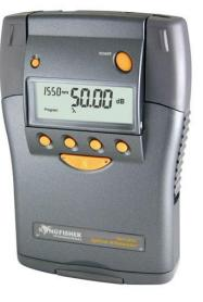
The KI 7010B series Automated Variable Optical Attenuator is an easy to use instrument for testing optical transmission equipment. It combines superb accuracy with high productivity.
