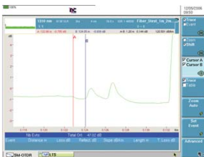
High resolution for detection of bends and close events
