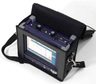
MTS/T-BERD 8000 platform with OTDR and OFI modules
