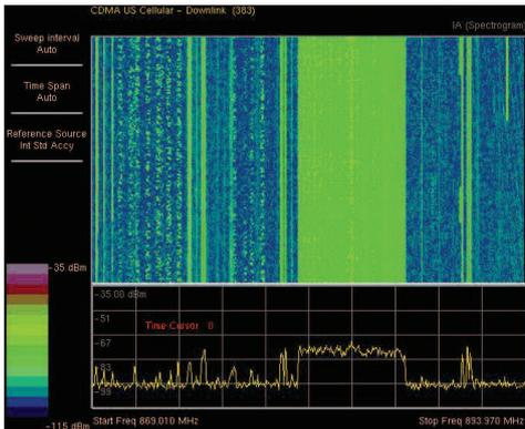
With Option 25, spectrogram measurements identifies intermittent interference.
