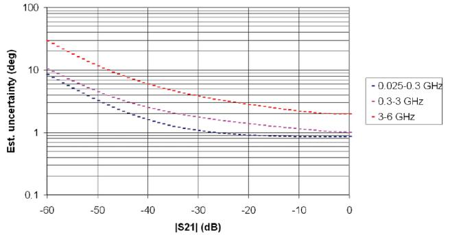
The uncertainty graphs above provide measurement uncertainty at 23° C after vector correction for the standard N connector type. Errors are worst-case contributions of residual directivity, source match, frequency response, network analyzer dynamic range, and connector repeatability. For the 1-path 2-port measurements, transmission tracking, crosstalk and physical load match termination was added. OSLN50-1 calibration components were used.
