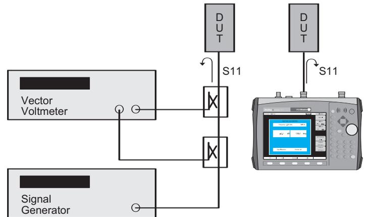
A side-by-side comparison shows how the VNA Master is a more convenient instrument for phase matching cables in the field.
