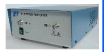
The 503L Broadband Amplifier is a rugged source of RF power suitable for a variety of UHF signal distribution and general laboratory applications. It is a compact fully solid state design. It features low-level intermodulation distortion and inherent protection against short and open circuit loads. The 503L amplifies the inputs of AM, FM, SSB, pulse and other complex modulations within its output and bandwidth capability.
