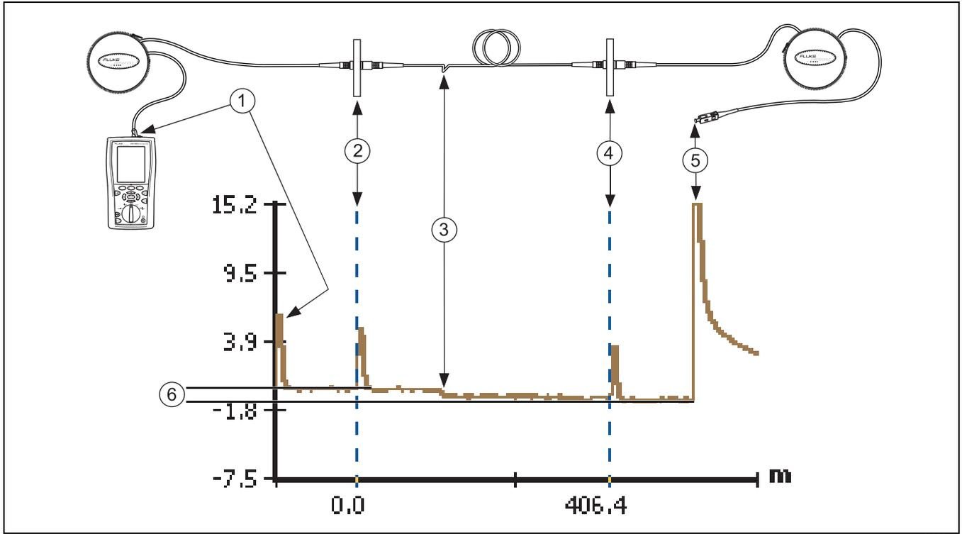
Figure 10. Typical OTDR Trace Features
