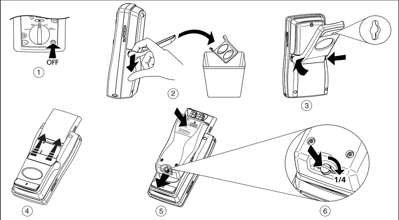
Figure 1. Installing the OTDR Module
