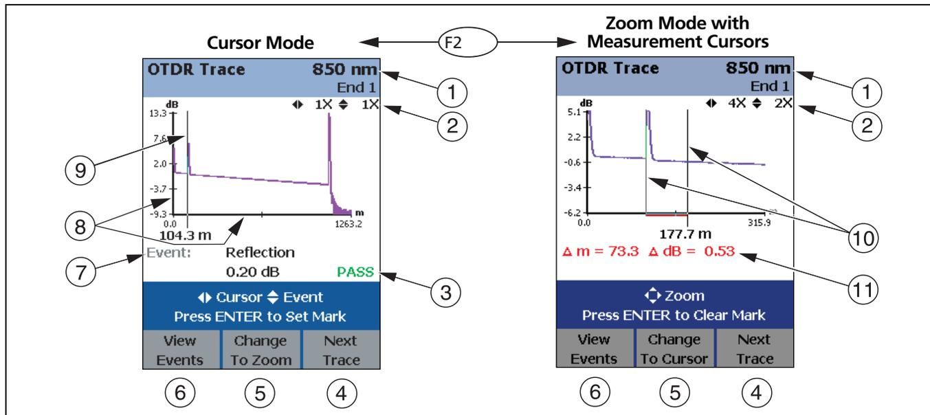
Figure 9. OTDR Trace Screens (launch compensation disabled)
