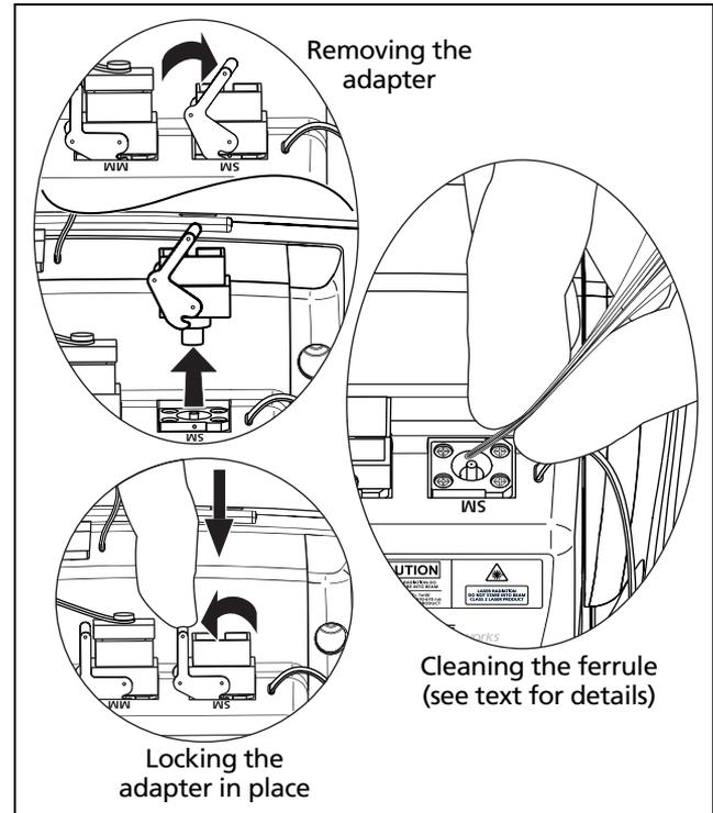
Figure 13. Cleaning the OTDR Ports
